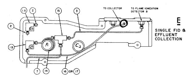
Receiver fitting (1A) is plugged. Column B effluent entering receiver fitting (1B) is split between restrictor A, (14), and effluent collection restrictor B<sub>2</sub>, (16), or C<sub>2</sub>, (17): The split ratio for restrictors B<sub>2</sub> and A (i.e., flow through restrictor
